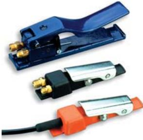
pneumatic and electric deadman controls are considered to be the most dependable and safest available in the industry. The pneumatic deadman control is a 3-way, normally closed valve, unlike a bleeder type that can cause accidental start up. The Schmidt electric deadman control has an epoxy sealed, normally-off switch that must be pressed to activate the blast system. A short-proof control option further protects against accidental start up, a leading cause of blasting injuries.
