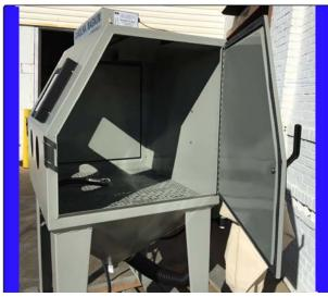
RECLAIMER: High performance 300 CFM cyclone type reclaimer separates good media from dust and by--products. GLOVE: Heavy duty cloth lined vinyl abrasive resistant snap-in gloves.
