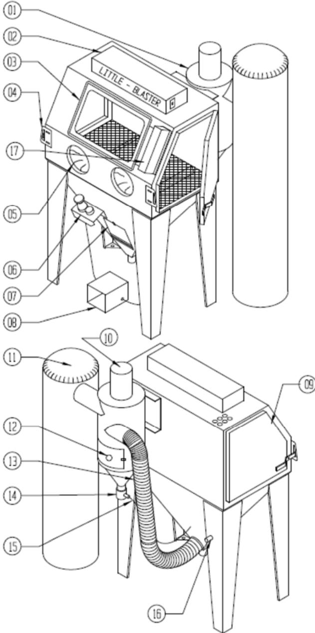
**1. Reclaimer:** High Performance 300 CFM cyclone type reclaimer separates good media from dust and by-products.
