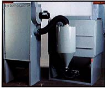
RECLAIMER AND D10 DUST COLLECTOR
