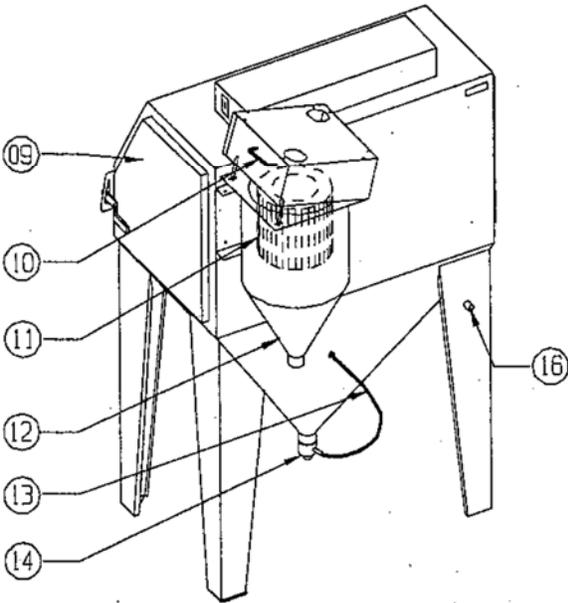
**1. Dust Collector:** 100 CFM cartridge type collector for better dust control providing cleaner working chamber.
