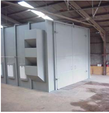
← BLAST ENCLOSURE FRONT / SIDE WORK DOORS AIR INLET LIGHTING
