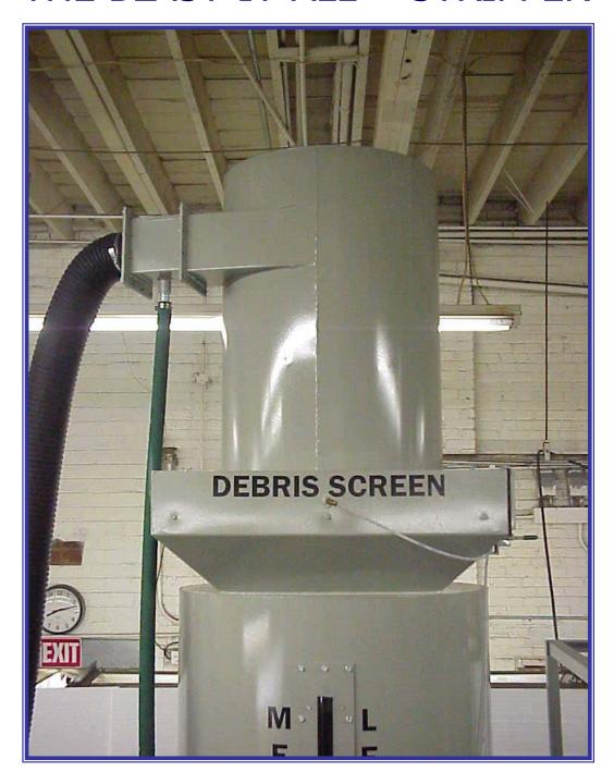
The reclaim is located on the top of the PMS unit above the debris screen. The media and dust is separated at this point. The dust and finer particles are rejected and transferred to the bag type dust collector. All media falls through the debris screen where larger paint chips and debris are collected. The reusable media then is directed to the media storage hopper above the pressure pot. A platform is provided for service and cleaning of the debris screen.
