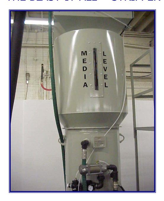
The media hopper has a sight gauge to show how much media is in the hopper. This helps prevent over filling of the unit that could waste or reject good media. The media hopper holds 1000 pounds of media that automatically refills into the pressure pot when the pot is depressurized.
