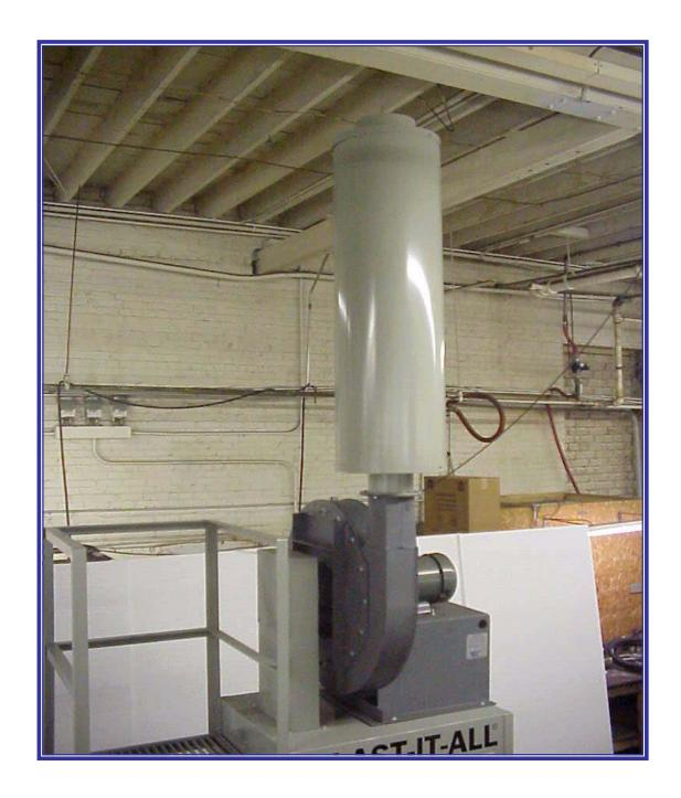
A high static fan rated at 900 CFM @ 20" WC is used to convey the blast media. The fan is driven by a 7 1/2 HP TEFC direct drive motor. On the outlet of the fan is a sound attenuater that is used to reduce the sound level.
